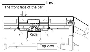
Adjust the radar if necessary. Small adjustments can be made by adjusting the radar to the radar mount plate position with using the fasteners in step 3.
